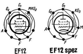
The Phædrus Audio EF12(*Spez*) is a drop-in replacement for the EF12 (or the EF12 *Spez*) tube in a wide variety of different circuits.
